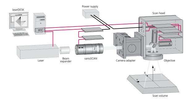
Galvanometer-driven scan heads first transformed laser systems into highly flexible processing tools. Their scope of functionality is closely tied to servo electronics and control concepts that satisfy diverse demands in dynamically positioning the laser beam and system monitoring.
